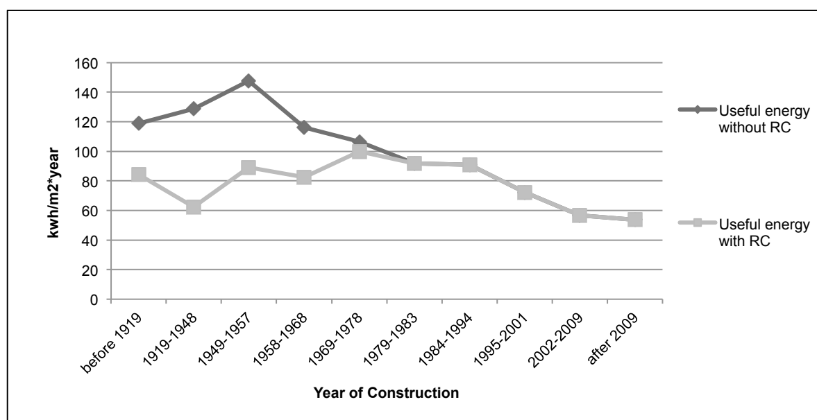
Figure 2. Useful energy of buildings according to construction year in kWh/m²*year (own elaboration based on own calculations with DESCoM).
