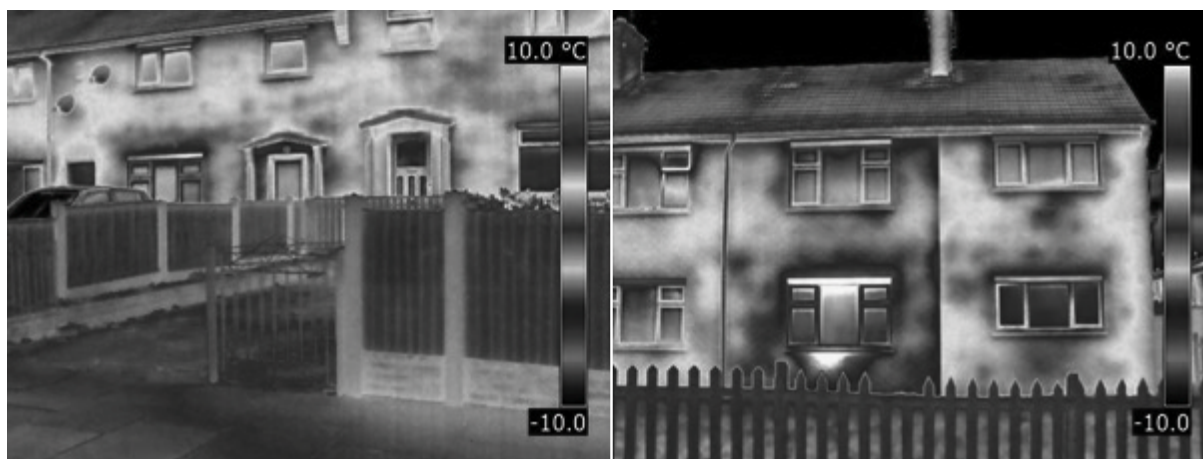
Figure 6. Thermal imaging of dwellings with cavity wall insulation showing the 'patchiness' of the wall insulation.
