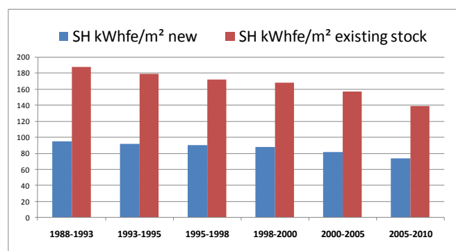
Figure 7. Comparison of evolution of unitary SH consumptions for new and existing dwellings ( kWh/m^2 , final energy, source: CEREN data).
