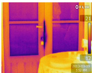
Figure 1. Thermal image showing a draught or cold air ingress entering the house from the join at two doors.
