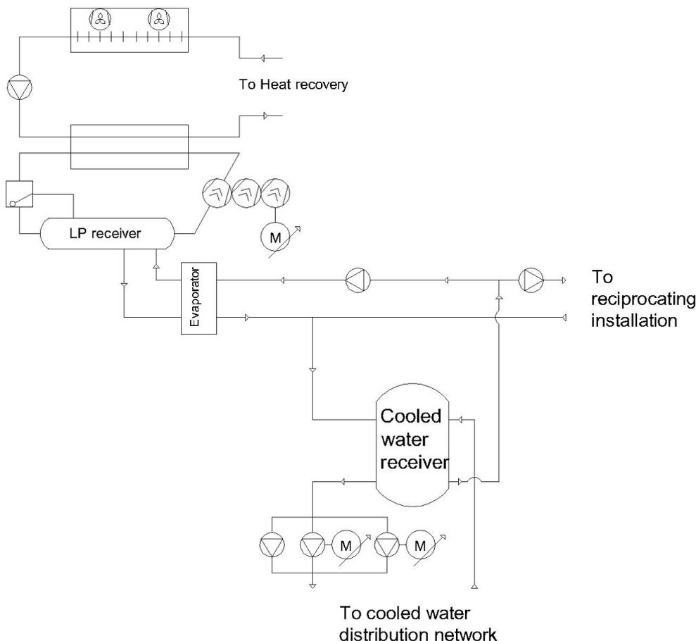
Figure 1. LDC Bourgogne refrigerating installation, screw compressors part.
