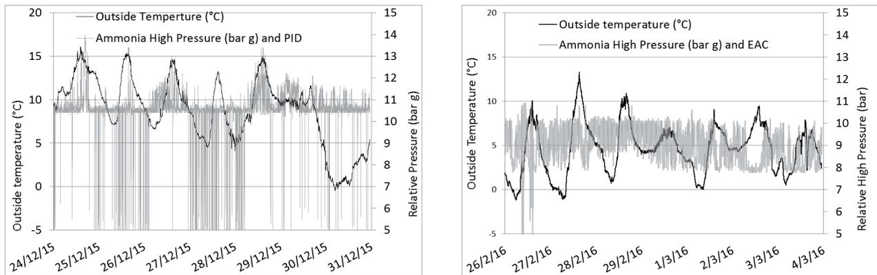
Figure 6. Outside temperatures and ammonia head pressure with PID (left) and EAC (right).
