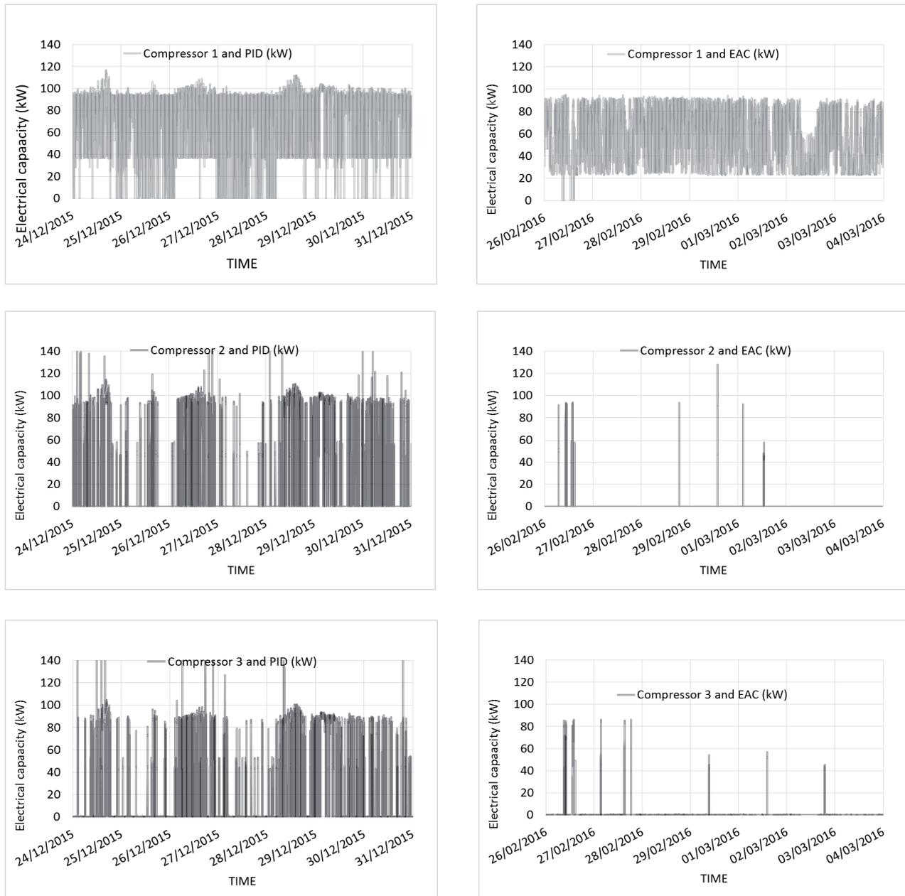
Figure 2. Compressors controlled with PID (left) and EAC (right).
