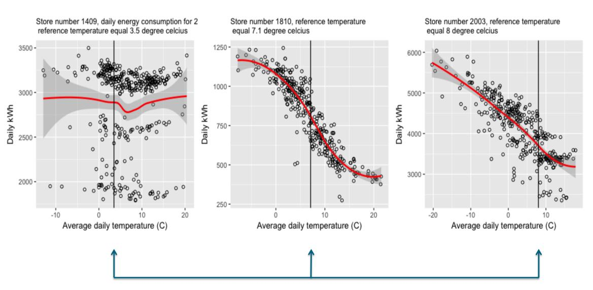
Example from three of the 132 stores, vertical line from PLR indicating the estimated changing point temperature (CPT)
