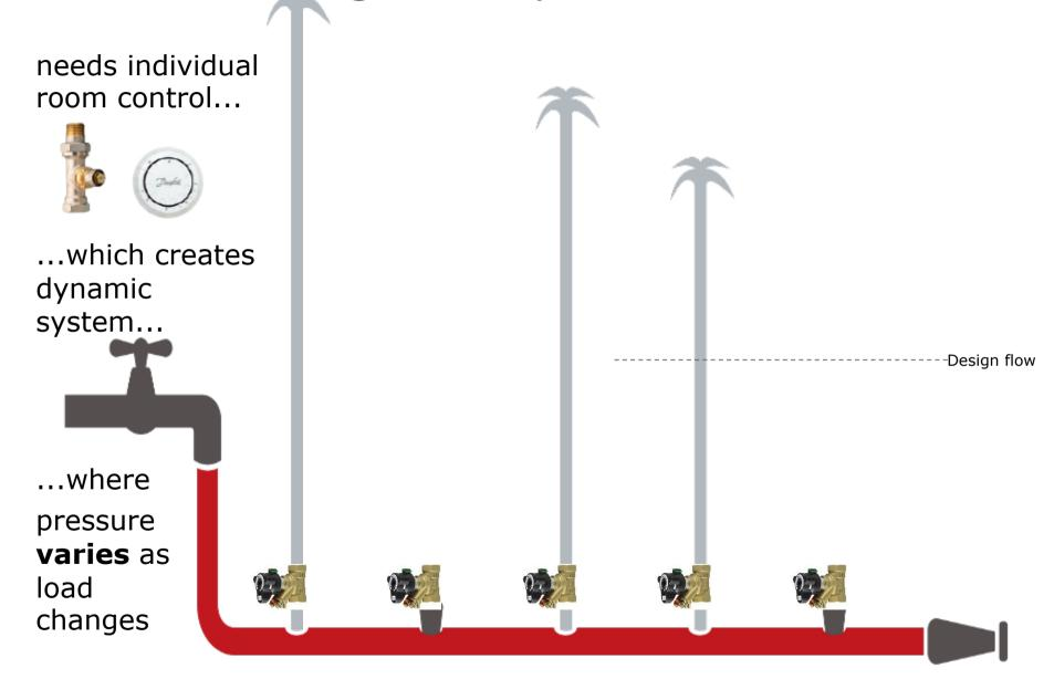
Dynamic balancing provides stable conditions at full and partial load...
