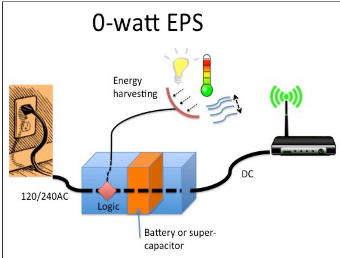
*Schematic illustrating how Standzero would be applied to an external power supply (EPS).*
