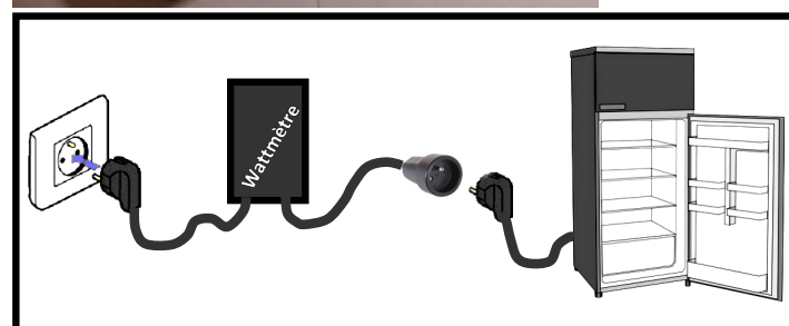
Figure 2. Picture of a serial wattmeter – datalogger used for the monitoring campaign.
