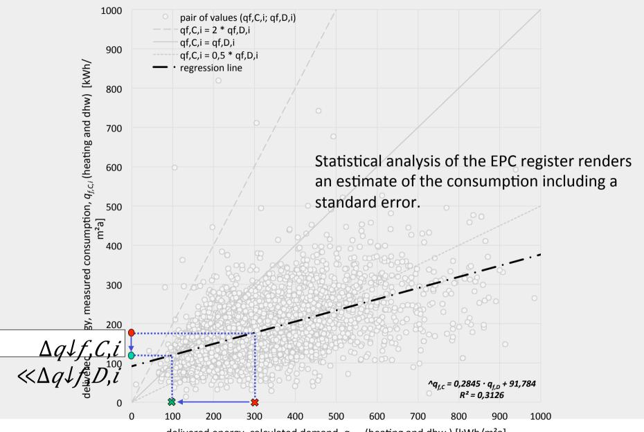
delivered energy, calculated demand,  $q_{f,D,i}$  (heating and dhw ) [kWh/m<sup>2</sup>a]
